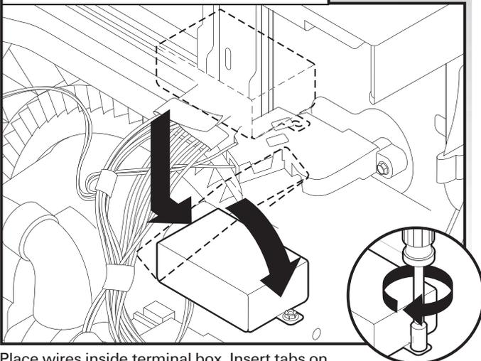
Place wires inside terminal box. Insert tabs on left side of cover. Make sure wires are tucked inside box. Close cover ensuring wires are not pinched. Use ¼" nut driver and previously removed screw to secure cover.
